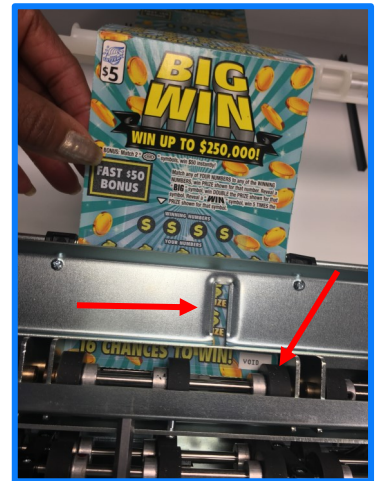
5. Feed past ticket sensor until touching burster rollers.
