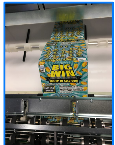
6. Tickets will be properly seated by burster.
