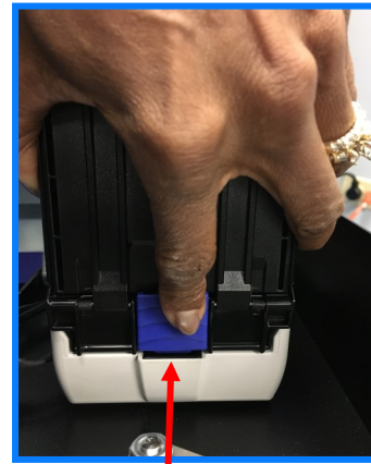
4. To release Cashbox from base, grab it and push up on the blue button.
